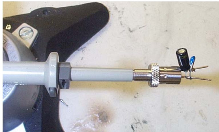
Figure 10 - Oscilloscope Probe with Probe Master 5125BA BNC Adapter. (Modified with wires for probe ground for ripple measurement, and two parallel decoupling capacitors added)
